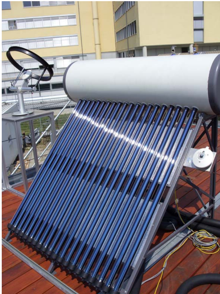
Abbildung 1: Foto des Systems TZ47/1500-20c während der Messung Picture of the system TZ47/1500-20c mounted on the test facility
